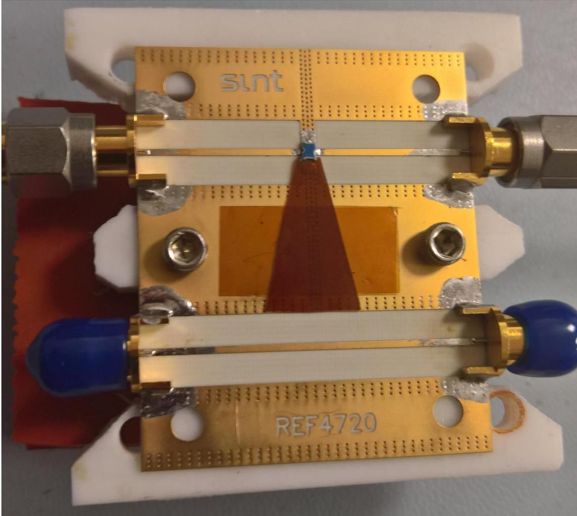
Figure 7: TT910.0SMT attenuator in the TT9-EVB modified to be a push-on RF Test Fixture.
