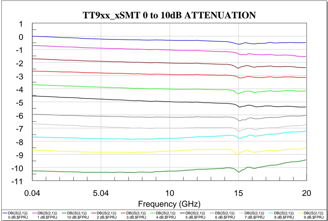
Figure 3: TS09xx.xSMT 0dB to 10dB Attenuation soldered devices on UTF fixture.
