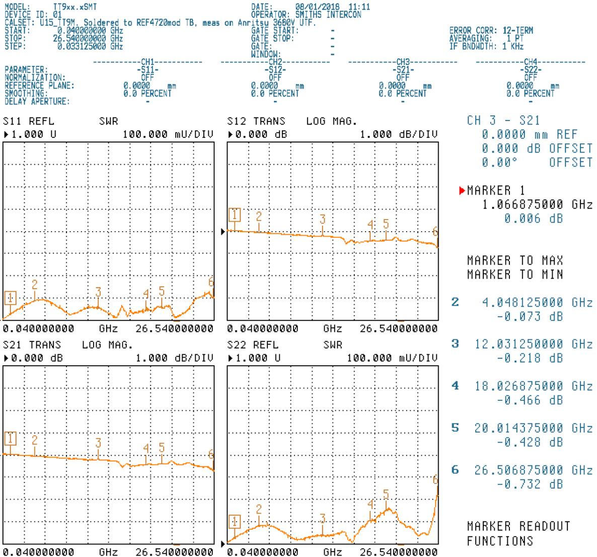
Figure 8: REF4720mod Test Board ThruLine measured on the Anritsu UTF.
