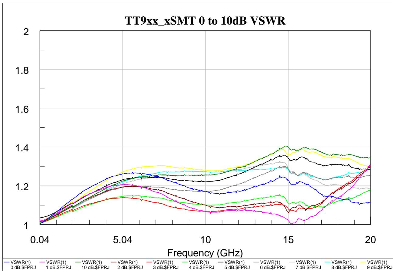
Figure 1:TS09xx.xSMT 0dB to 10dB VSWR soldered devices on UTF fixture.
