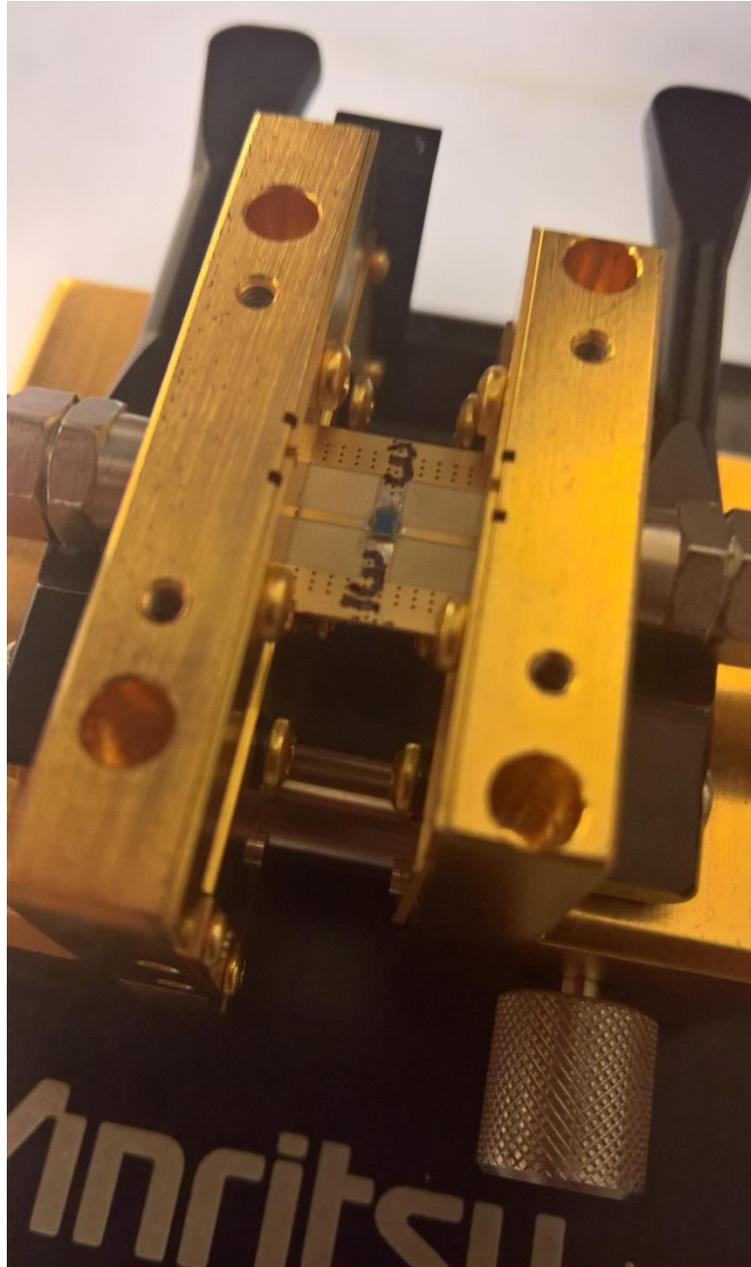
Figure 5: TT903.0SMT soldered to REF4720 mod Test Board being measured on the Anritsu 3780 UTF.
