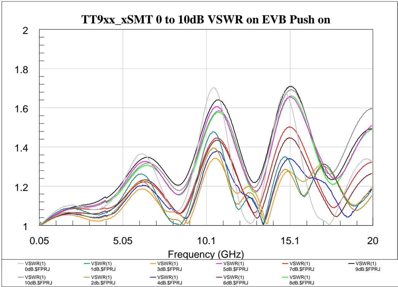
Figure 2: TS09xx.xSMT 0dB to 10dB VSWR on EVB push-on fixture.
