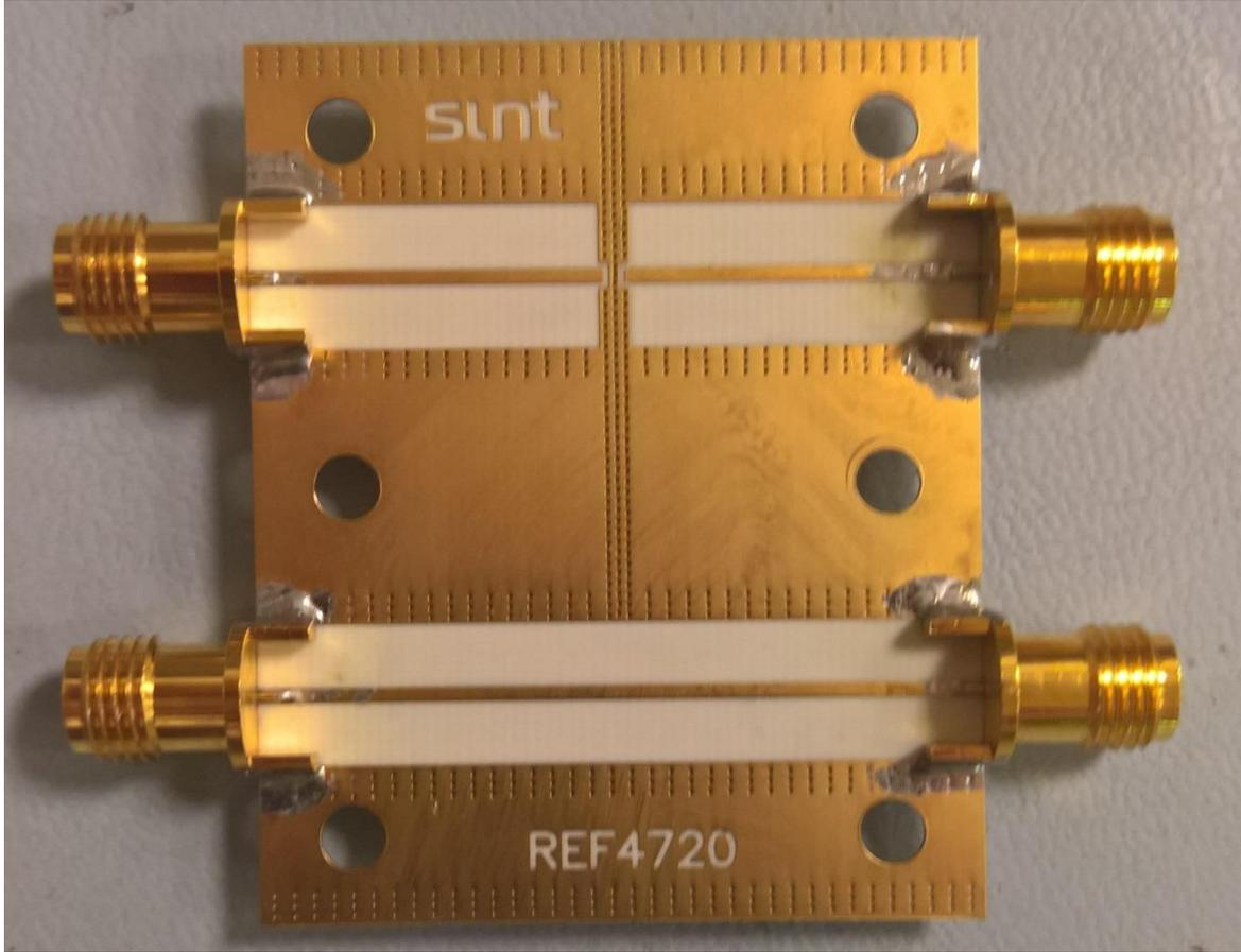
Figure 6: TT9-EVB is the TT9XX.XSMT attenuator family Customer Evaluation Test Board, which consists of the REF4720 Test board and the 009-01-078 Edge launch connectors.
