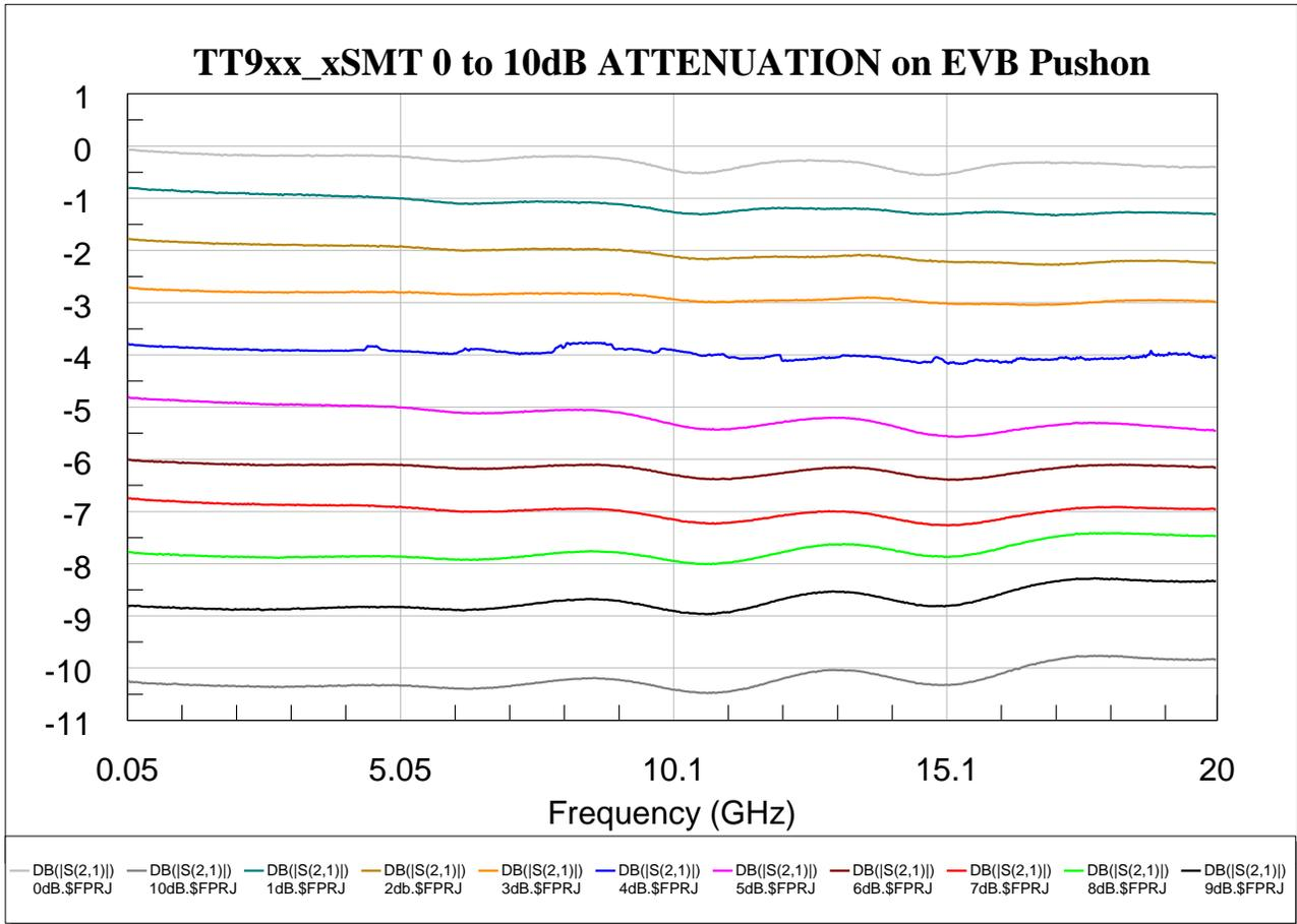
Figure 4: TS09xx.xSMT 0dB to 10dB Attenuation on EVB push-on fixture.
