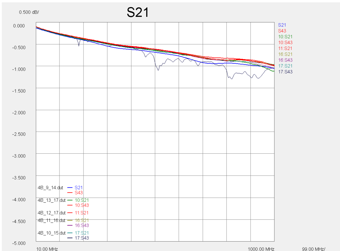
Figure 19: Insertion Loss VS Frequency Overlays Measurements of 4B Configurations with Entire Test Setup
