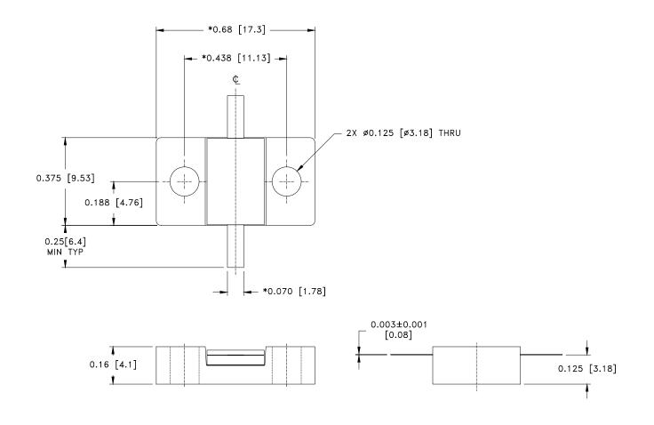
ALLOW ±0.010 ON TOP PLATE FOR MISALIGNMENT. \* DIMENSIONS TO BE SYMMETRICAL ABOUT C.L. WITHIN ±0.005.
