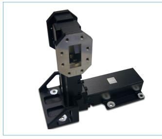
The X-Band WR112 high-power isolator is designed for use in the 8-8.5 GHz range for TWTA applications for communications and TT&C. It boasts an interesting flight heritage deep space programs including missions to Mars and Mercury and shortly on the Juice mission to Jupiter. These devices exist in several variants ranging from 100W to 180W CW. The use of low emissivity paint is a requirement of the originating user.
