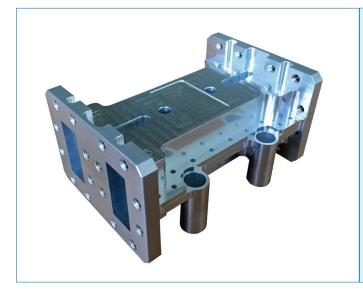
The WR112 2x2 hybrid couplers are designed as a power splitter or combiner with their function and power handling capacity dependent on how they are used and whether one of the ports is suitably terminated. This item is arranged so that the coupling is between the broad walls and boasts substantial flight heritage in LEO missions. Broad-wall coupling is employed to make a more compact product.
