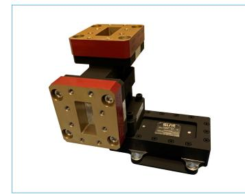
The X-Band WR112 high-power isolators were designed to be used in the 8.35 to 8.5 GHz frequency range and used on the output of a deep space transmission system. It has substantial flight heritage and was qualified for the harshest of space environments. The use of low emissivity paint is a requirement of the originating user.
