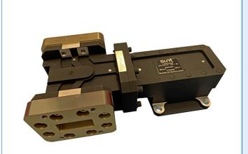
The X-Band WR112 high-power isolator was designed to be used in the 8.3 to 8.5 GHz frequency range for data link and TT&C communications. It boasts an interesting flight heritage and has been used on missions to Mars and Mercury. These devices exist in several variants ranging from 100W to 180W CW. The use of low emissivity paint is a requirement of the originating user.
